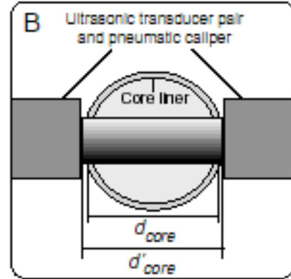
Transducer-receiver 500 kHz 2 $\mu$ sec pulse
