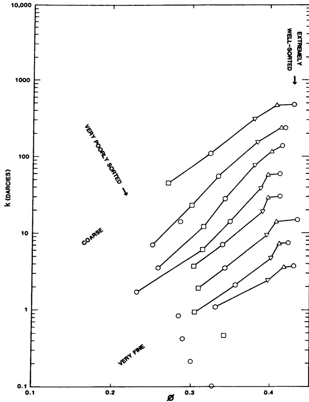
Figure 15.2 Permeability-porosity data from unconsolidated artificial sand packs by Beard and Weyl (1973). Symbols distinguish sorting groups; lines connect grain size ranges. (Nelson, 1994)
