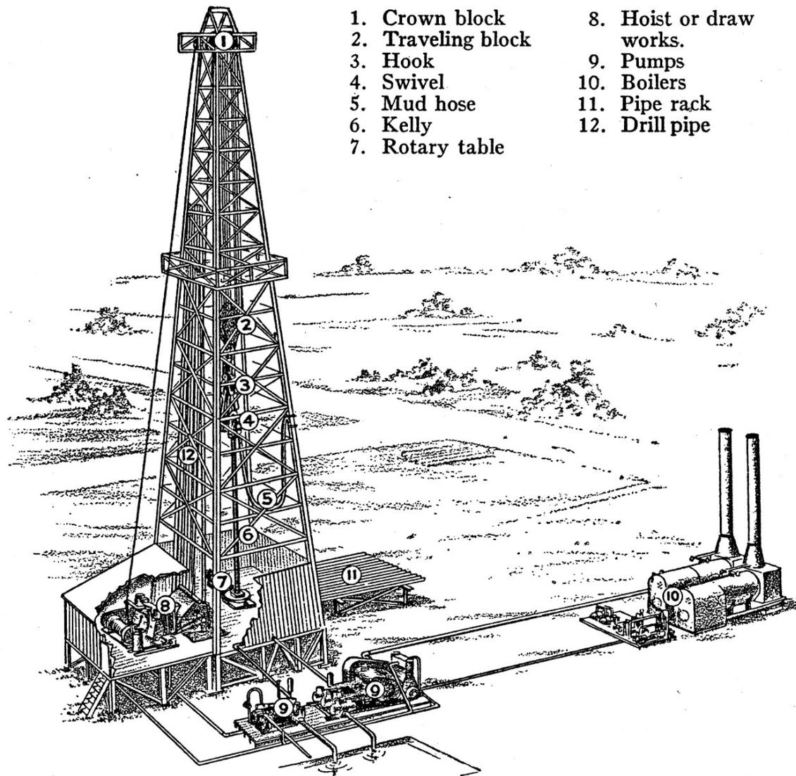
Rotary drilling bores a hole by rotating a bit on the end of a string of pipe, called drill pipe, some of which is shown standing in the derrick ready to be "run in" to the hole. The draw works at the left is the mechanism that runs most of the job. The pumps in the foreground force mud down through the drill pipe and back up between the drill pipe and the wall of the hole, flushing out the cuttings and plastering the wall of the hole so that it will not cave.
