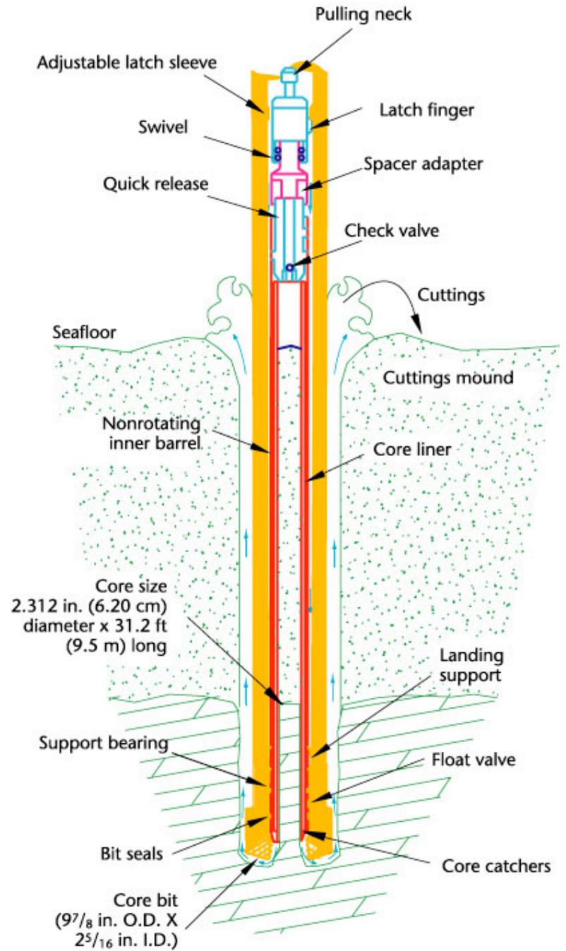
When the operator wants to know the exact character of the rocks he is drilling he uses a core barrel and takes a core which his geologist or micro-paleontologist or micro-mineralogist or chemist can study. When he wants to divert his hole from the vertical he uses a whipstock or knuckle joint.
