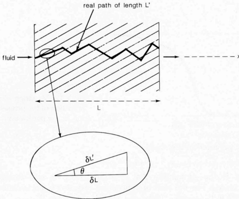
Fig. V.13. Notion of tortuosity:  $L'$  is the real flow path of the fluid and  $L$  is the apparent path.  $\tau = \frac{\delta L'}{\delta L} = \frac{L'}{L}$ .
